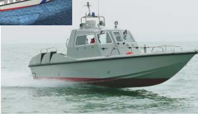
From Conceptual Design to Final Commissioning: Halmatic Cougar Enforcer 33 Patrol Boat. Twin HJ274 waterjets
